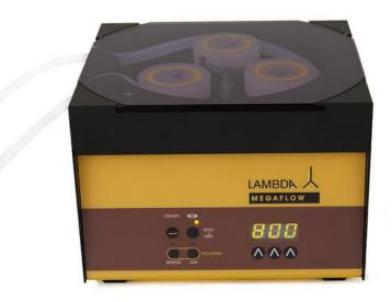
MEGAFLOW is a specially designed laboratory peristaltic pump for long term continuous processes with increased flow rates of up to 60'000 ml/hour. High precision, reproducible and long term stable flow rates are achieved with the quartz driven BLDC motor and unique tubing compression technique in the large pump head.
